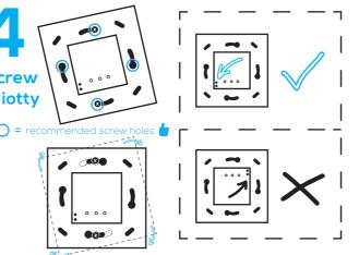
Push all the wires back into the wall box and try to allow as much space for the switch as possible. (Do not push the wires using the back of the switch). Insert the iotty Smart **Shades Switch** in the wall box screws. Position the switch so that the buttons are located at the bottom.
