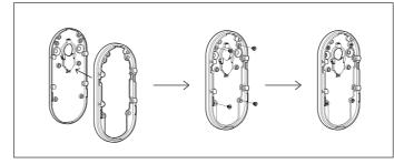
(EN) Place the Retrofit Extender onto the mounting plate and secure it with four screws.
