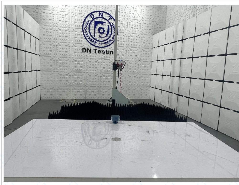
Radiated Emission Test View(Above 1GHz)
