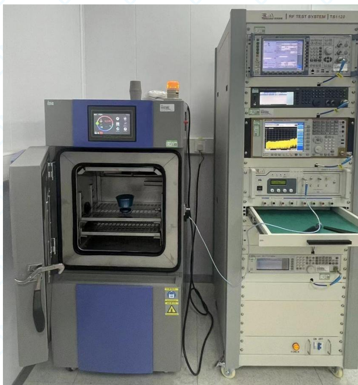
Setup for Transmitter & Receiver Spurious Emissions
