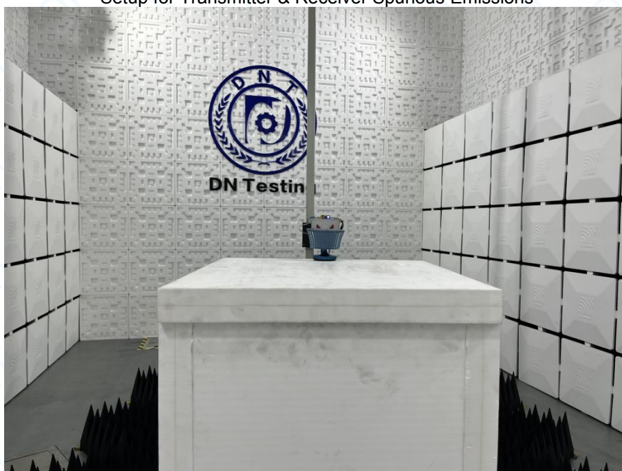
Setup for Transmitter & Receiver Spurious Emissions
