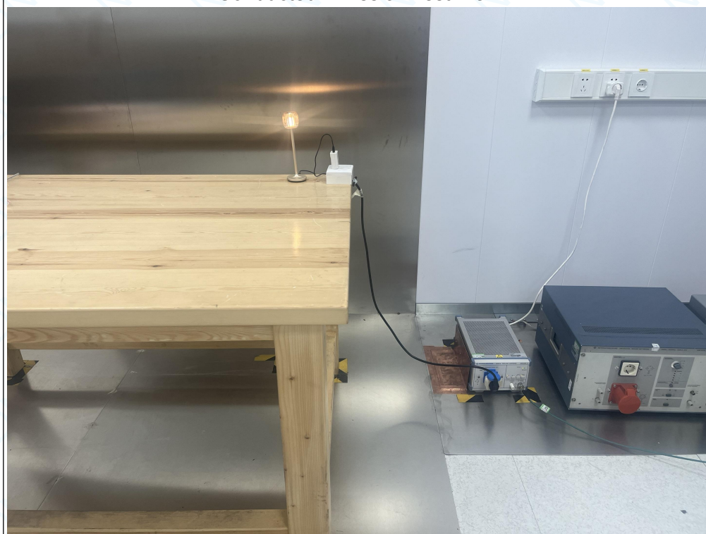
Conducted Emission Test View
