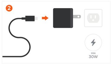
Connect the included USB-C charging cable to a power adapter (not included).
