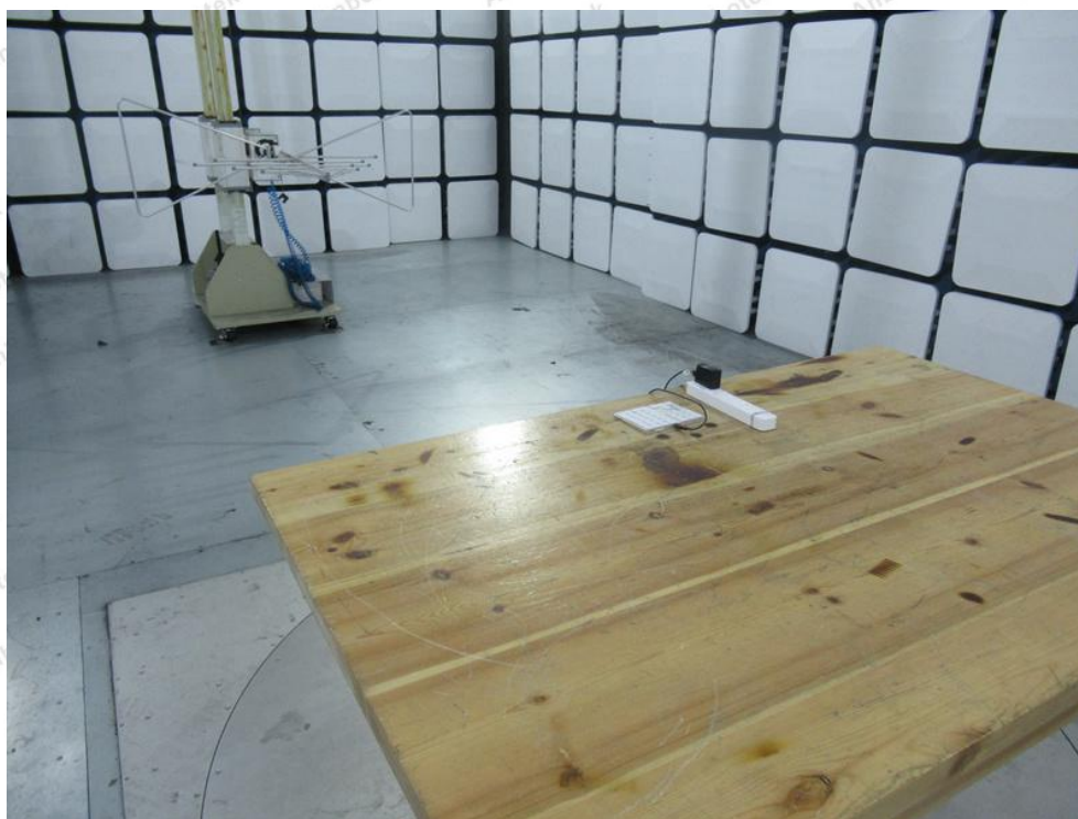
Photo of Radiation Emission Test
