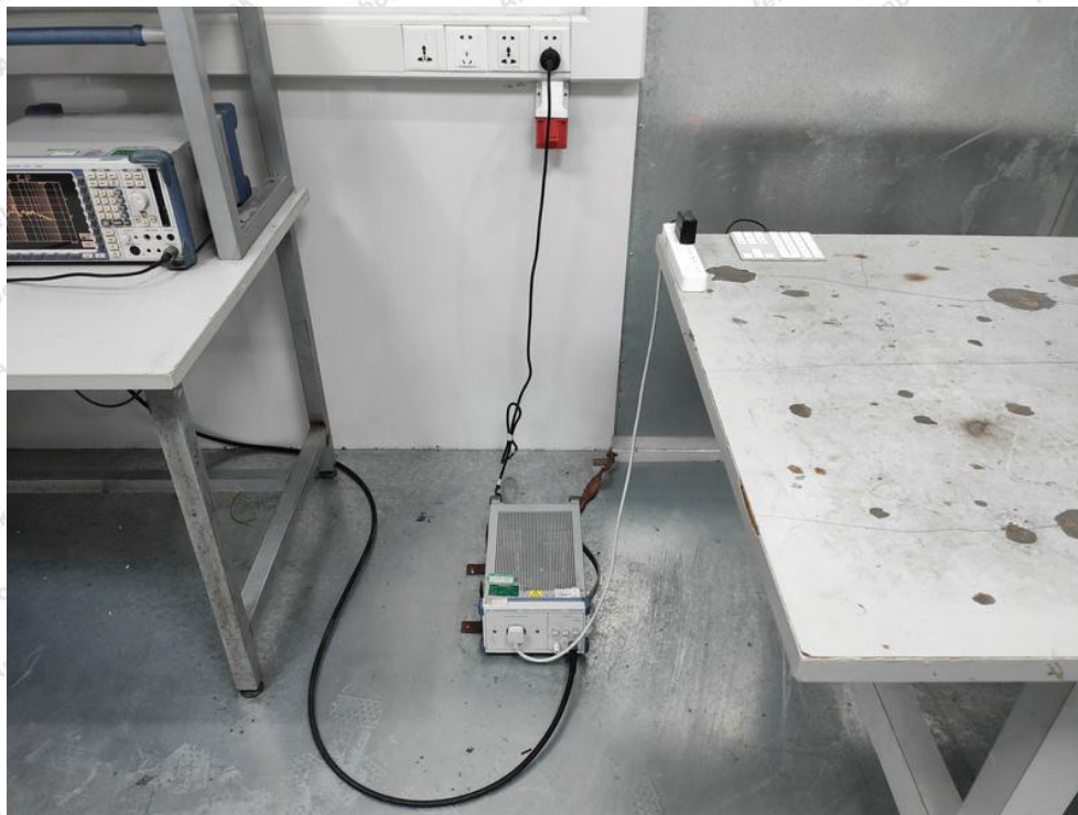
Photo of Conducted Emission Test
